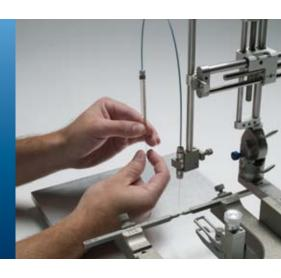
Many delicate neuroscience, stem cell and chemical dispensing applications require the use of pulled glass needles, also known as glass capillary needles, or PEEK tubing with precision syringes, as opposed to stainless steel needles. Properly attaching a pulled glass needle or a length of PEEK tubing to a syringe is difficult, and the traditional use of wax or other workarounds often exposes the experiment or technique to inaccuracy or contamination.
